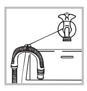
If it is place over the edge of a basin or sink be sure the free end of the hose should not be underwater.
